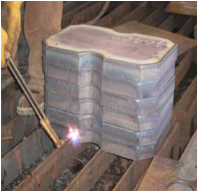
Figure 5. Manually post heating.
